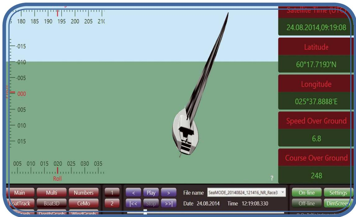
The SeaMODE™ Speed Lab Software collects the data from the SeaMODE™ MD100 motion detectors, processes the data and presents its as graphical information. Shown here is one of the many dashboards available to choose from.
